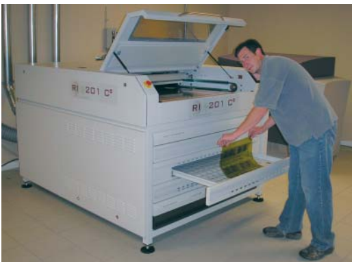
Ben Sadler removes a plate from the washout section.
