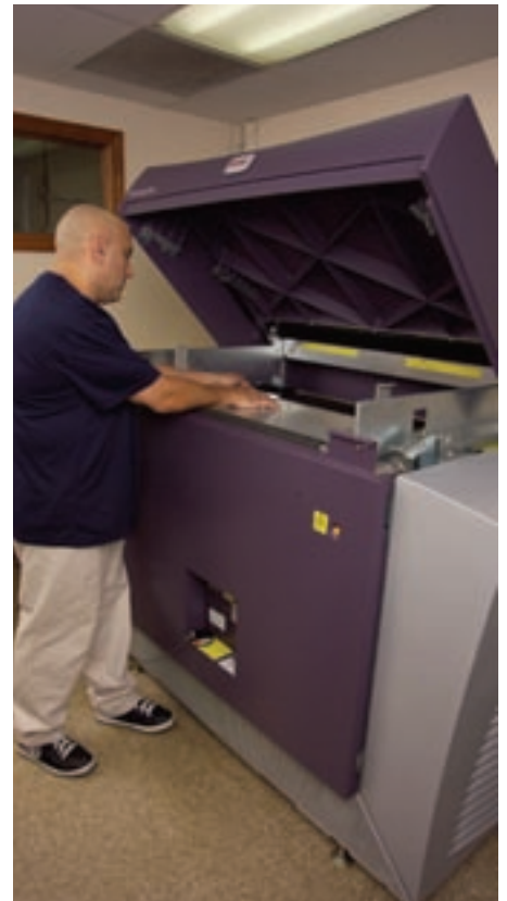
Carmen Demaio positions a plate for imaging on the Kodak Thermoflex Narrow platesetter.
